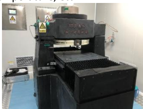
Figure 1. (Ultra-precision flycutting machine tools)
