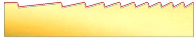
Figure 3. Cross-sectional profile of Fresnel lens with tool path compensated with the tool nose radius offset, as shown in red.
