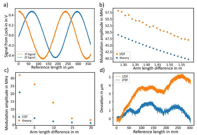
**Figure 2.** a) Sine and cosine signal detected by the Lock-ins and deviation of length measurement. b) and c) Modulation amplitude changes depending on the arm length difference d) Deviation of length measurement to reference
