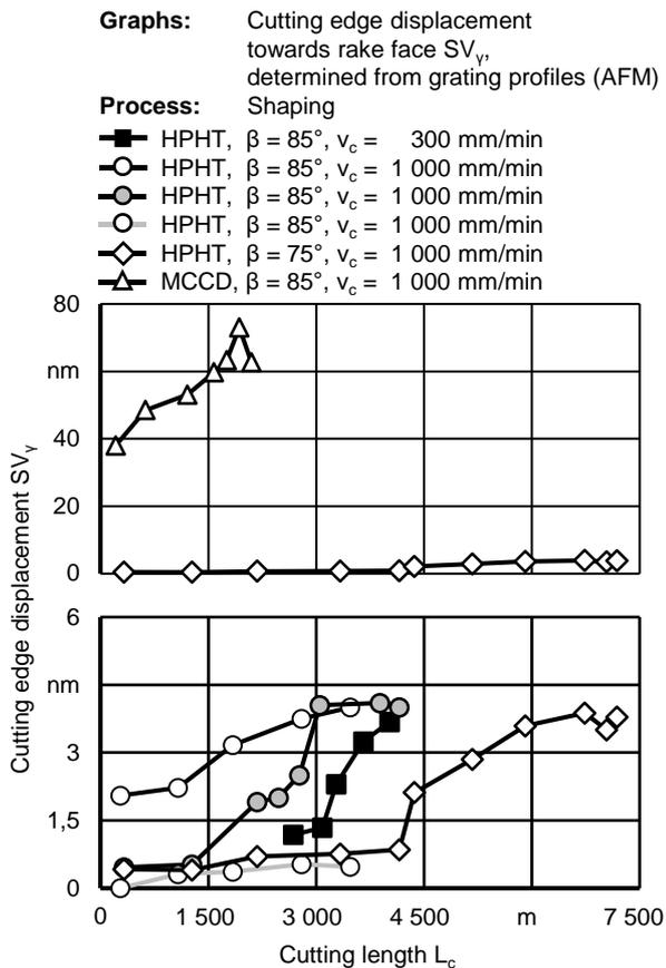
**Figure 6.** Cutting edge displacement towards rake face  $SV_\gamma$  in dependence of cutting length  $L_c$  for various diamond tools
