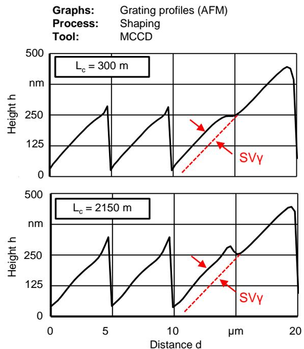
**Figure 5.** AFM-profile measurement of diffraction grating with  $1 \mu\text{m}$  grating
