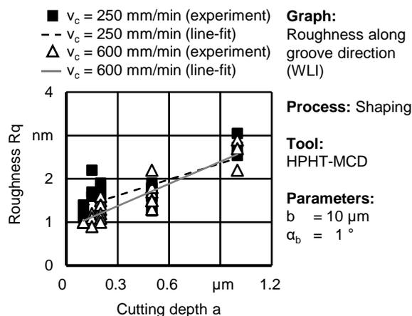
**Figure 4.** Roughness  $R_q$  in shaped Ni-P-Structures for various cutting depths  $a$
