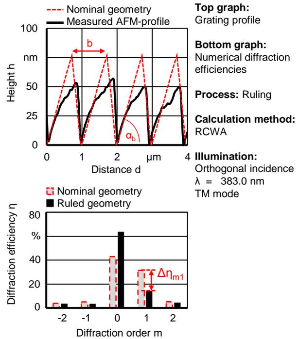
**Figure 2.** Ruled Ni-P-Grating and corresponding calculated diffraction efficiencies
