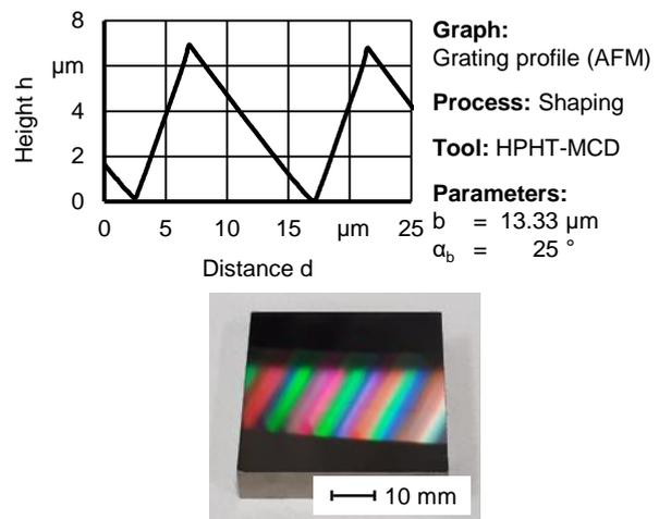
**Figure 7.** Echelle grating in Ni-P
