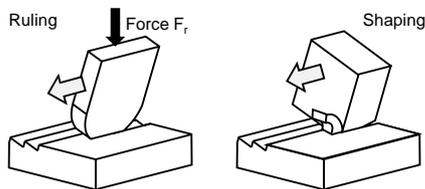
**Figure 1.** Ruling and shaping (schematic)
