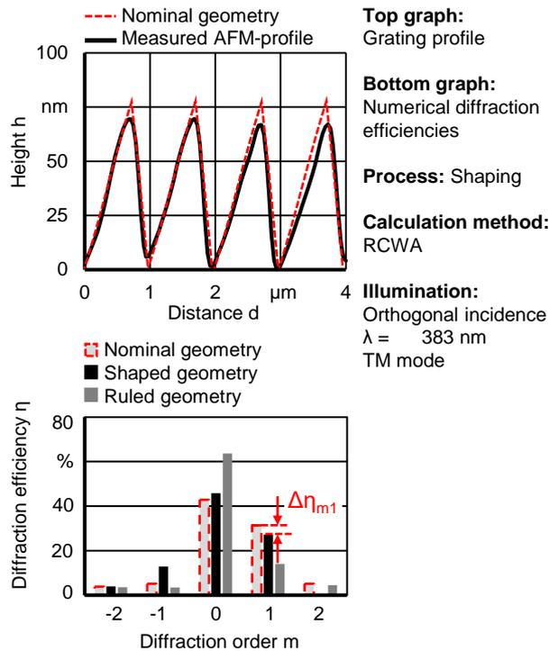
**Figure 3.** AFM-profile measurement of diffraction grating with  $1 \mu\text{m}$  grating period
