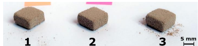
Figure 2. Cuboid test specimens manufactured with BJ technology using 85% peach kernel and 15% PVA powder mixture.
