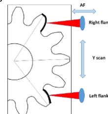
Figure 1. Gear profile measurement strategy
