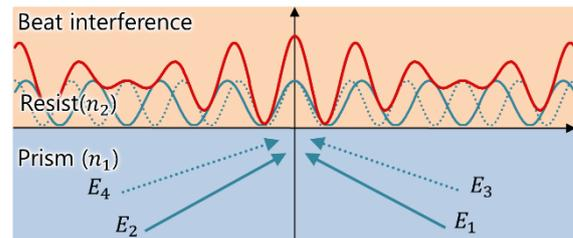
Figure 1. Schematic of spatial beat of evanescent wave interference
