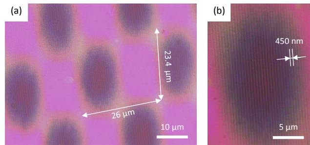
**Figure 5** Microscopy image of fabricated structure
