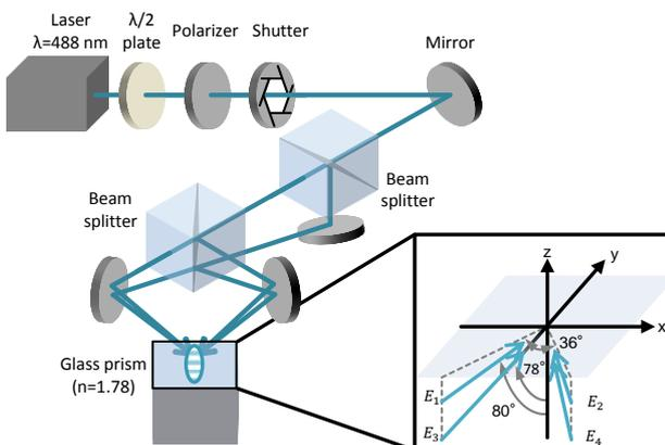
**Figure 3** Setup of fabrication experiment
