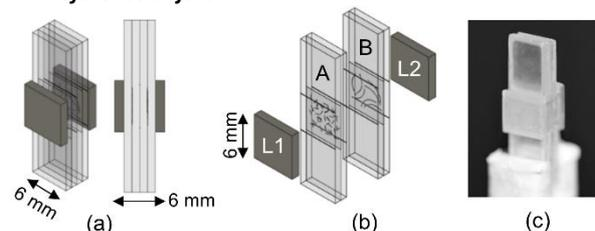
**Figure 1.** Dismountable reference object: (a) Schematic representation of the object in the assembly state; (b) exploded view showing the two fiber-reinforced polymeric layers (L1 and L2) and the sub-samples A and B containing the calibrated fibers; (c) picture of the reference object.
