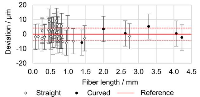
Figure 3. Deviations between measured fiber lengths and corresponding calibrated values for straight and curved fibers. The dashed red lines are positioned in correspondence of the expanded calibration uncertainty  $\pm U_{cal}$ .
