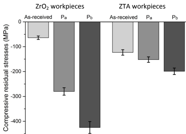
Figure 6. Residual stresses of the as-received and ground ZrO 2 and ZTA workpieces (machined with P a and P b conditions) measured through XRD technique.
