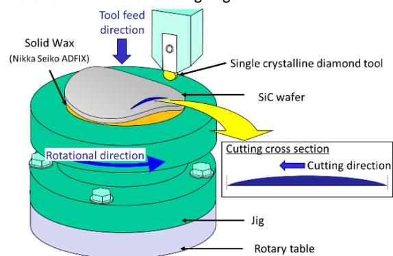
Figure 1. Schematic of experimental apparatus
