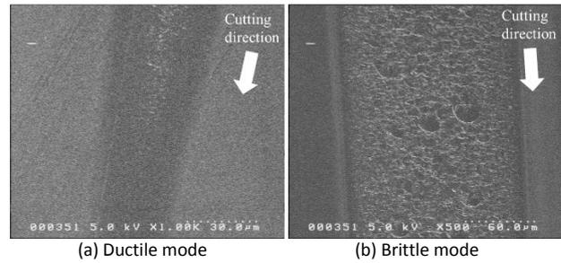
Figure 3. SEM images of ductile and brittle surfaces of machined SiC (Tool 2,  $v=30$ m/min)
