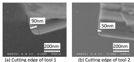
Figure 2. Cutting edge radius of diamond tools
