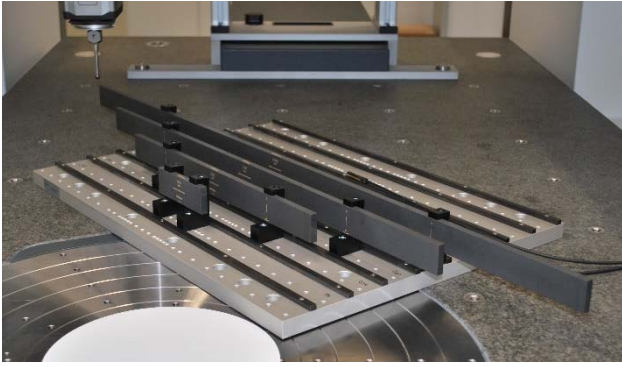
Figure 5. Set-up of four gauge blocks made of ZeroCera™ (100 mm to 1000 mm) placed diagonally in the measurement volume of the CMM.
