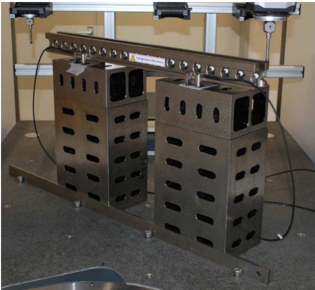
Figure 2. Set-up of the steel-made step gauge in diagonal orientation and in 0.4 m height.
