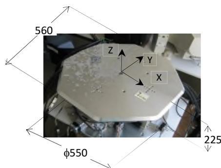
Figure 1. Redundant Parallel Positioning Table Device (Rd-PPTD)
