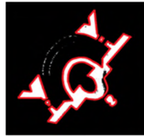
Figure 2. Comparison between nominal shape (red contour) and observed geometry for local defect detection
