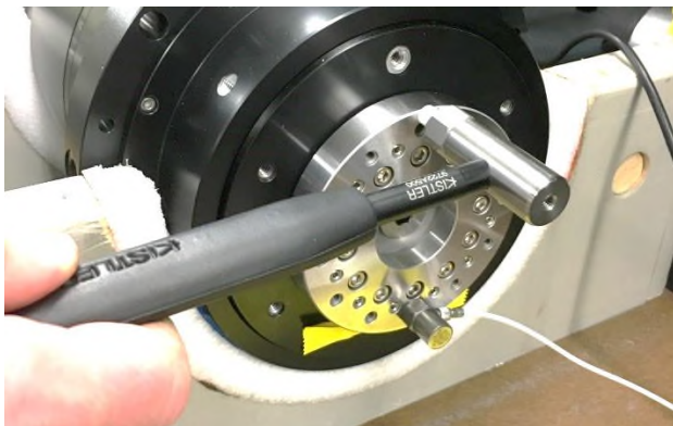
Figure 4. Modal impact test in the axial direction
