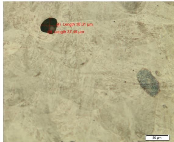
**Figure 4.** Material microstructure with a visible pore
