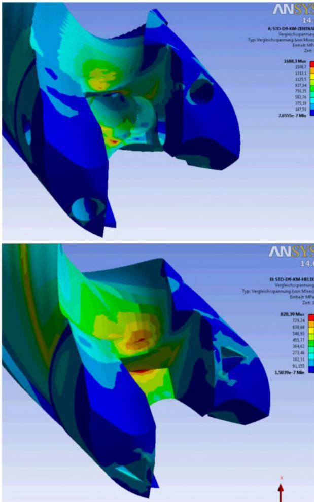
**Figure 3.** Example of FEM analysis of the inner stresses in the conventionally fabricated (upper) and 3D-printed drill base body
