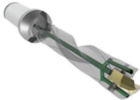
Figure 1. Coolant ducts in the conventionally fabricated drill base body
