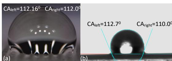
**Figure 4.** Water droplet on micro textures with Serial No. 7 (Table 1) and height 50 µm (a) by developed setup (b)
