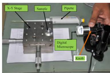
**Figure 3.** Contact angle measurement setup
