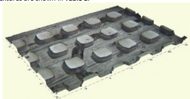
Figure 2. Micro textures fabricated by DXRL
