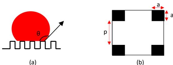
Figure 1. (a) Contact angle (b) Unit cell containing four micro textures (top view)
