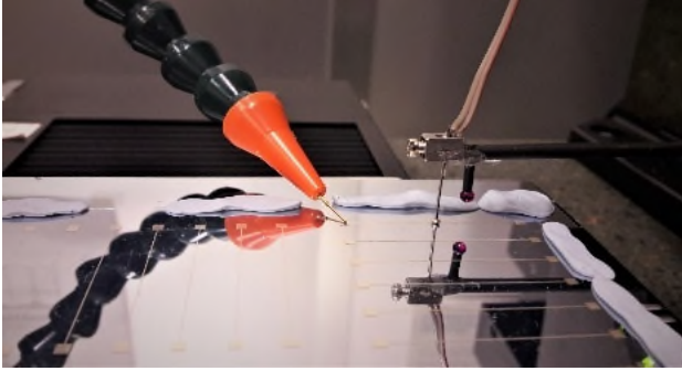
Figure 3. The reference (fixed) electrode (left) and the moving electrode (right).
