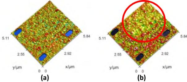
Figure 1. Measured surface before and after shot peening showing the slots acting as relocation landmarks and the shot peened region (b – red circle).
