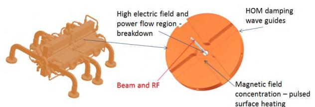
**Figure 1.** CERN CLIC structure with indication of the functional features that demand surfaces to be machined by Ultra Precision Technology techniques.
