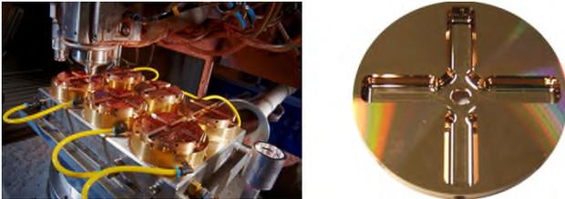
**Figure 2.** Diamond milling of an Ultra High Precision machined copper cavity for high gradient normal conducting accelerator of CERN CLIC. Diameter of the disk is 80 mm and the shape of the entire product is within 2  $\mu\text{m}$ , with a surface roughness of 5 nm Ra in the zone around the central iris and 25 nm Ra elsewhere in the cross-shape. Rotational symmetric surfaces are machined by turning, while non-rotational symmetric surfaces are milled.
