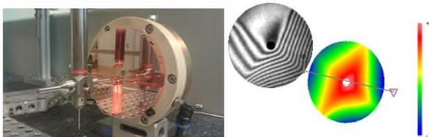
**Figure 3.** Cern CLIC disk on the CMM and flatness measurements on a white light interferometer.
