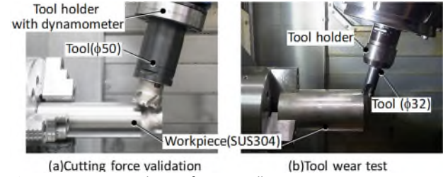
Figure 4. Experimental setup for turn milling test
