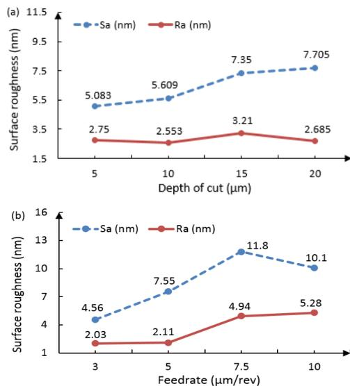
**Figure 2.** The machined surface roughness against: (a) depth of cut while the feedrate kept at  $3 \mu\text{m}/\text{rev}$ ; (b) feedrate while depth of cut kept at  $10 \mu\text{m}$ .
