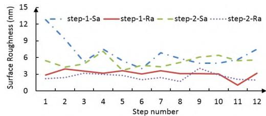
**Figure 4.** The surface roughness of machined micro steps
