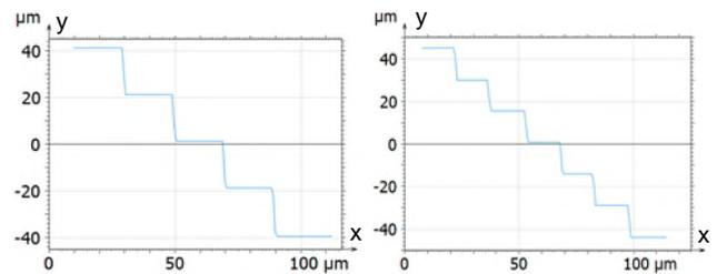
**Figure 3.** Cross-sectional view of machined micro step features  $20 \times 20 \mu\text{m}$  (left) and  $15 \times 15 \mu\text{m}$  (right)
