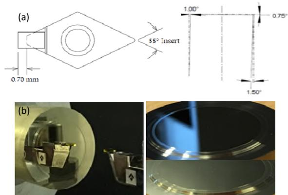
Figure 1. (a) The geometrical design of the facet diamond cutting tool and (b) the nanometric cutting setup and fabricated samples.
