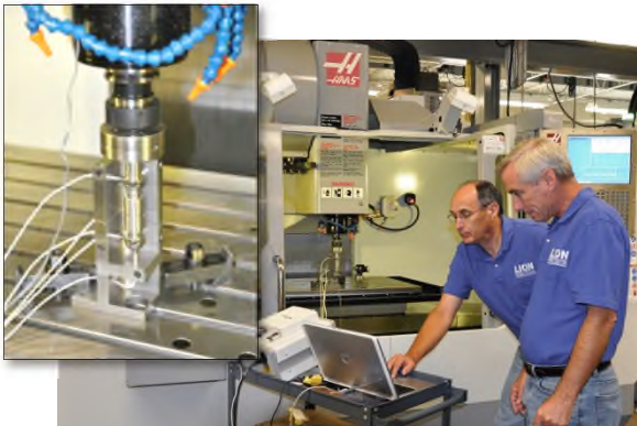
Figure 2. Complete spindle error motion measurement using five capacitive sensors with nest, double-ball artifact, and spindle error analyzer. Photo courtesy of Lion Precision.
