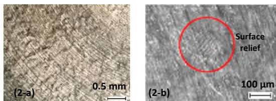
**Figure 2.** Optical micrograph of the finished surface after face turning (a) and enlarged image of the surface relief (b)
