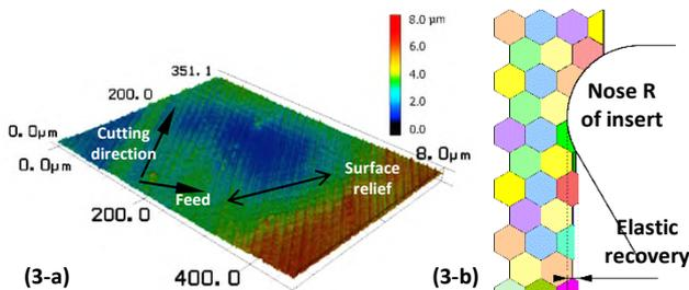
**Figure 3.** Laser microscopy contour image of the finished surface (a) and a schematic showing the effect of crystal anisotropy after face turning (b)
