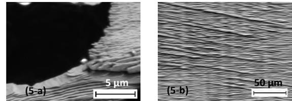
**Figure 5.** SEM micrograph of the chip edge (a) and surface relief caused by stress-induced martensite on the free chip surface (b)
