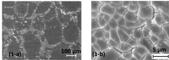
**Figure 1.** Optical micrograph of a mechanically polished surface (a) and SEM micrograph of a chemically polished surface (b)
