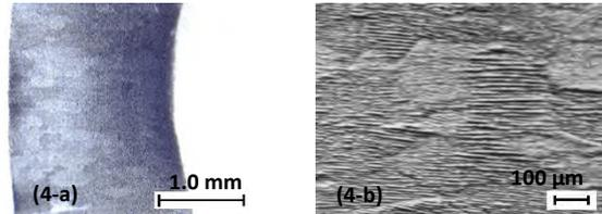
**Figure 4.** Optical micrograph of the free chip surface (a) and enlarged SEM micrograph (b)
