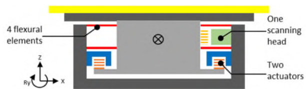
Figure 1. 1-dof architecture relying on flexural elements
