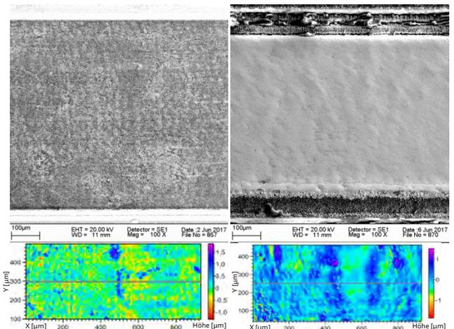
**Figure 2.** Surface roughness of the measuring chamber area before (left) and after (right) laser polishing
