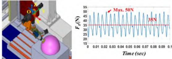
**Figure 4 3D view (left) and machining force (right) in simulation**
