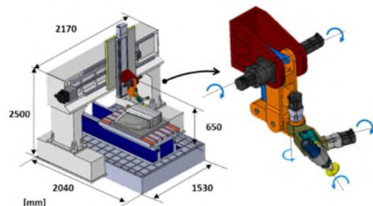
Figure 1 Conceptual design of robo-finishing machine
