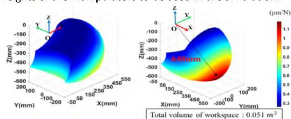
Figure 2 Maximum compliance for an arbitrary force in workspace
