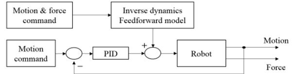
**Figure 6 Servo control process (top), and PID-based feedforward control (bottom)**
