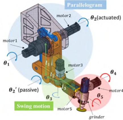
**Figure 3 Conceptual design of manipulator**
