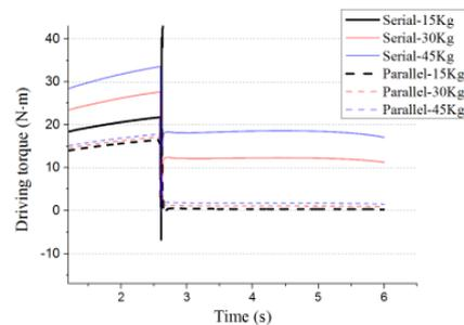
**Figure 7 Simulation result of abrupt change when entering workpiece (driving torque of motor 2)**
