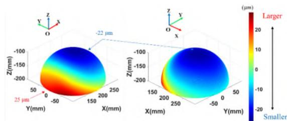
**Figure 5 Magnitude of total error when machining hemisphere (Normal force: 50N)**
