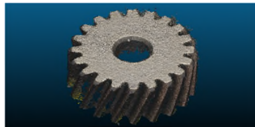
Figure 1. 3D point cloud of a 21.8 mm radius gear produced by photogrammetry
