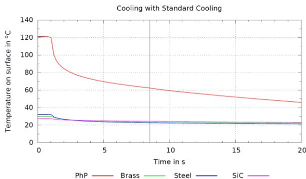
Figure 3. Cooling of the surface of the insert with standard cooling. Ejection of the moulded part after 8.5 s.
