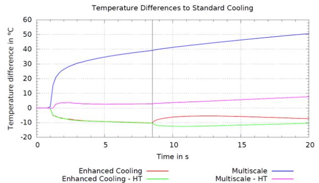
Figure 4. Difference to standard cooling of PhP inserts.
