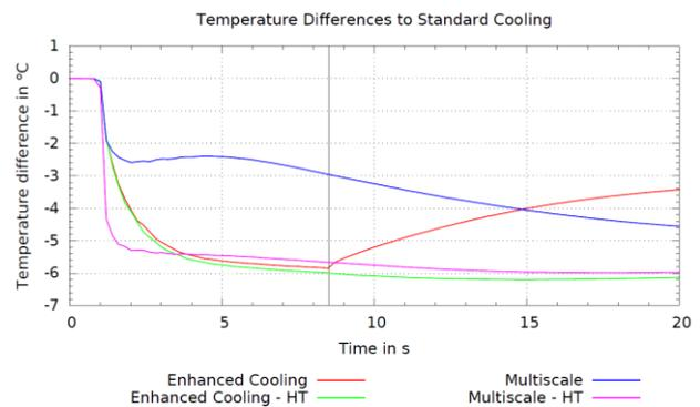
Figure 5. Difference to standard cooling of brass inserts.
