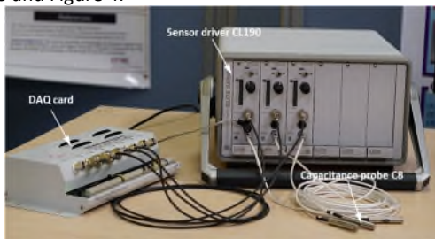
Figure 3. Kinematics error measurement device
