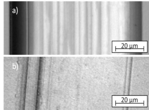
**Figure 4.** a) UP-turned silicon surface  $R_q = 9\ \text{nm}$ . b) Machined Zerodur surface  $R_q = 11.2\ \text{nm}$ .
