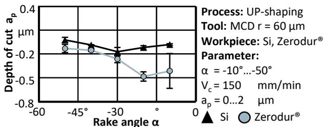
**Figure 1.** Influence of variation of the rake angle  $\alpha$  on the maximum depth of cut  $a_{p,\text{max}}$ .
