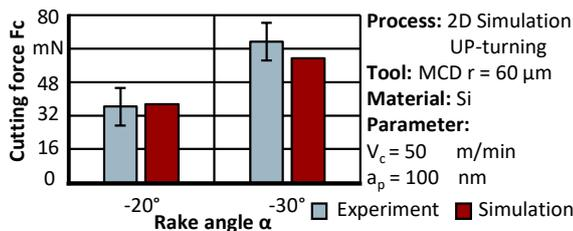
**Figure 2.** Influence of the rake angle on the cutting force  $F_c$  for Si while UP-turning of silicon and 2D simulation results.
