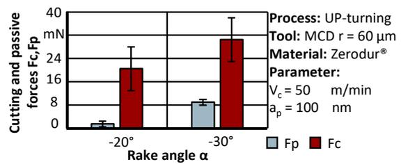
**Figure 3.** Influence of the rake angle on the cutting force  $F_c$  and  $F_p$  for Zerodur® UP-turning.
