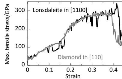
**Figure 6.** The maximum tensile stress of lonsdaleite in the [1100] direction and diamond in the [110] direction
