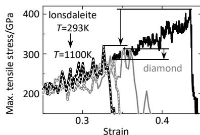
**Figure 5.** Thermal stability of lonsdaleite in the [0001] direction and diamond in the [111] direction at temperatures of 293 K and 1100 K
