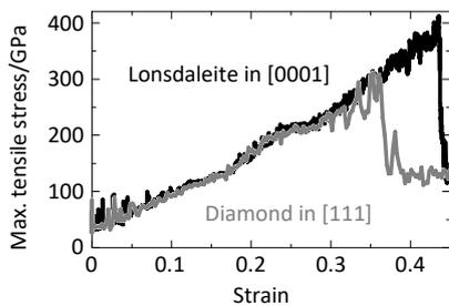
**Figure 4.** The maximum tensile stress of lonsdaleite in the [0001] direction and diamond in the [111] direction
