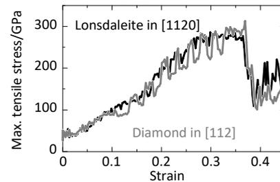
**Figure 7.** The maximum tensile stress of lonsdaleite in the [1120] direction and diamond in the [112] direction
