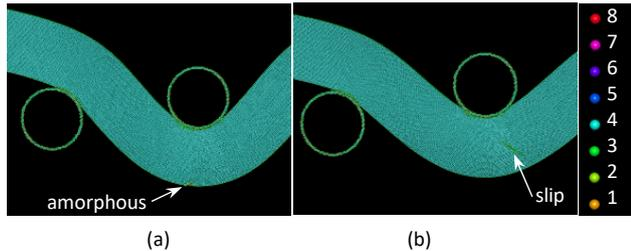
**Figure 2.** Different fracture mechanism (a) an amorphous phase transformation from the surface in lonsdaleite (b) a slip on the (100) plane in the bulk in diamond
