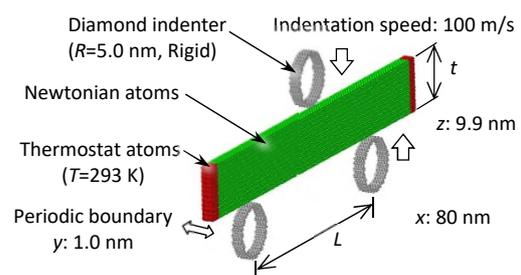
Figure 1. Initial model for three-point bending
