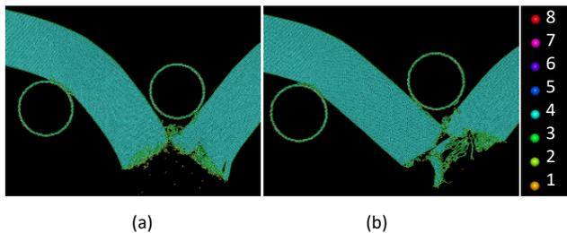
**Figure 3.** After crack extension (a) lonsdaleite (b) diamond
