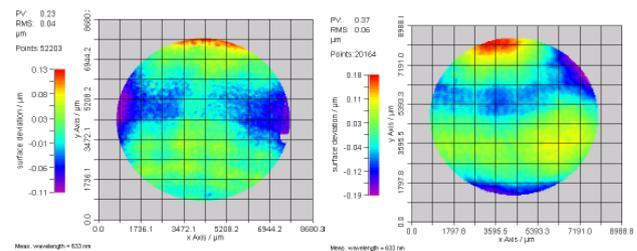
**Figure 2. Fisba form measurements a) cavity number one form and b) COC lens at 90 bar holding pressure from cavity number one**
