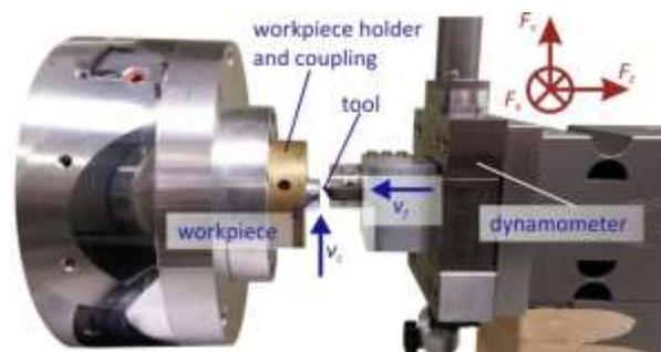
Figure 1. Experimental setup of the performed plunge-cutting process
