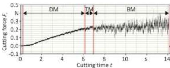
Figure 4. Cutting force along the  $\langle 2-1-10 \rangle +15^\circ$ -direction with a cutting speed of 10 mm/min
