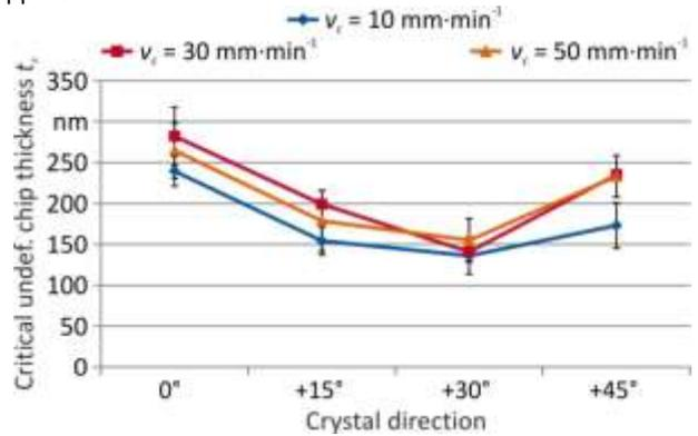
Figure 5. Critical undeformed chip thickness during plunge-cutting in different crystal directions
