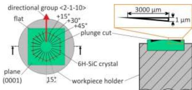
Figure 2. Plunge-cutting scheme of a 6H-SiC single crystal specimen
