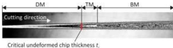
Figure 3. Machined plunge-cut along the  $\langle 2-1-10 \rangle +15^\circ$ -direction with a cutting speed of 10 mm/min
