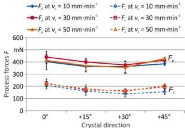
Figure 6. Process forces during cutting in different crystal directions within the transition mode (TM)
