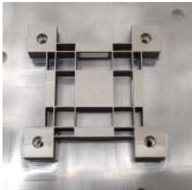
Figure 3 The HS-AFM stage. Stage size 70\ \text{mm} \times 70\ \text{mm} , mirrors for optical interferometers not shown.
