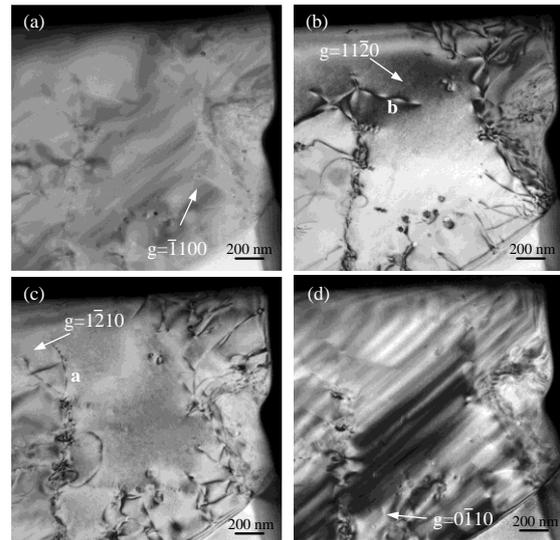
**Figure 3.** TEM BF images in two-beam conditions of dislocation underneath 6H-SiC particle (a)  $g=[-1100]$  (b)  $g=[11-20]$  (c)  $g=[1-210]$  and (d)  $g=[0-110]$ .
