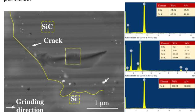
Figure 1. SEM image and EDS spectra of fractured surface morphology.
