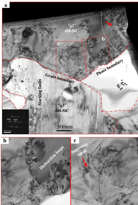
**Figure 2.** (a) Cross-sectional Bright field (BF) TEM image of the subsurface damage beneath fracture area (b-c) high magnifications corresponding 'b' 'c' marked in (a), respectively.
