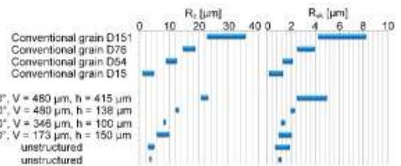
Figure 4. Comparison of the achieved workpiece roughness between conventional honing stones (D151 - D15) and the novel CVD diamond honing stones
