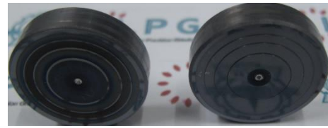
Figure 5. SiC fabricated by only laser ablation (left) and "laser + ultra-precision grinding chain" (right)
