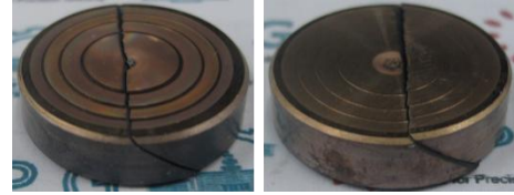
Figure 6. 45^\circ cross-sectioned surface of SiC workpiece for subsurface damage observation
