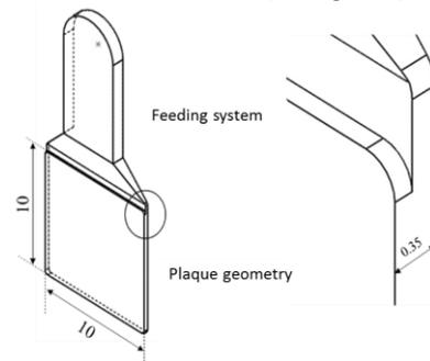
Figure 1. Thin-walled plaque geometry (all dimensions are in mm).
