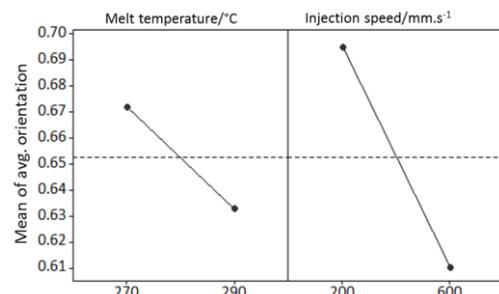
**Figure 3.** Main effect plots of melt temperature and injection speed for fiber orientation in flow direction.
