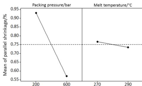
**Figure 2.** Main effect plots of packing pressure and melt temperature for the shrinkage in the flow direction.
