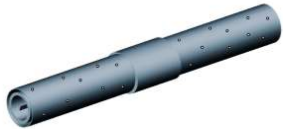
Figure 2. Test object resembling roundwood, built from an elliptic cylinder accompanied by two round tubes and a gauge. (nominal diameter 250 mm, overall length 2 m).
