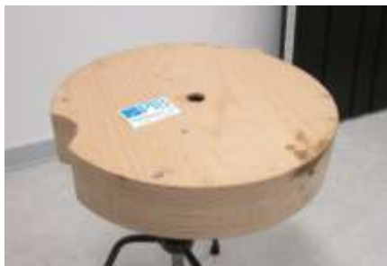
Figure 1. Disc made from veneer laminate to characterize the influence of surface colour and subsurface scattering in fringe projection measurements (nominal diameter 500 mm, thickness 100 mm)
