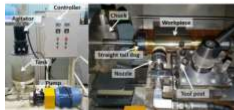
Figure 2. Configuration of the fluid jet polishing system
