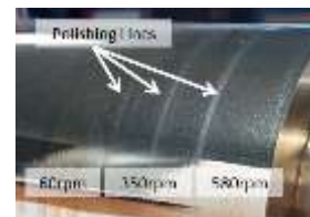
Figure 8. Polishing lines were generated by FJP along the roll surface
