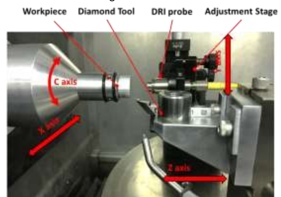
Figure 1. On-machine measurement system configuration
