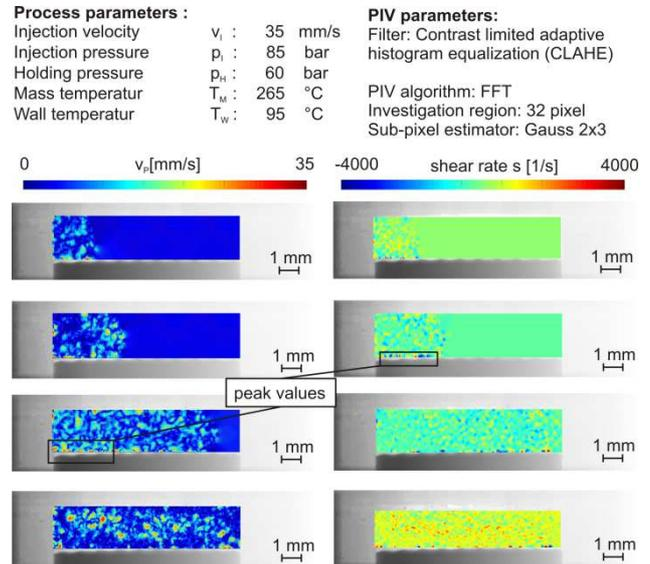
**Figure 2.** Velocity and shear rate distribution, determined by x-ray PIV
