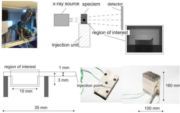
**Figure 1.** Experimental setup and schematic representation of the examined cavity
