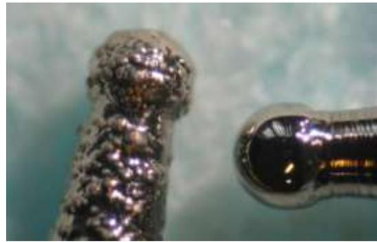
**Figure 4.** (left) NiP-coated and (right) finished specimen, diameter of spheres approx. 1 mm.
