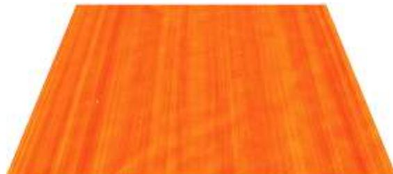
**Figure 6.** 3D view of a CLSM measurement of the concave cylinder, cylinder subtracted, size  $279 \mu\text{m} \times 250 \mu\text{m} \times 264 \text{ nm}$ . Roughness:  $S_a = 3.0 \text{ nm}$ ,  $S_q = 3.9 \text{ nm}$ ,  $S_z = 264 \text{ nm}$ .
