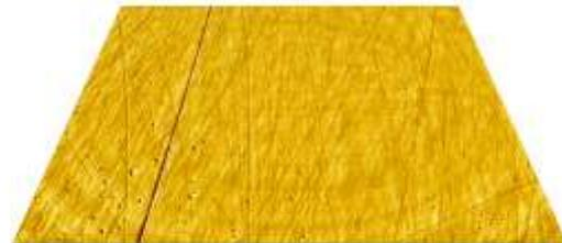
**Figure 5.** 3D view of a CLSM measurement of finished sphere (sphere subtracted) before FIB,  $100 \mu\text{m} \times 99 \mu\text{m} \times 87 \text{ nm}$ . Roughness:  $S_a = 3.2 \text{ nm}$ ,  $S_q = 4.9 \text{ nm}$ .
