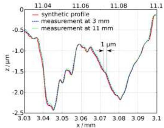
Figure 5. Simulated profile (red solid curve: eroded with template, dilated with circular tip as a structuring element) in comparison with the measured profile at two intervals of 8 mm distance (blue and green dashed curves).
