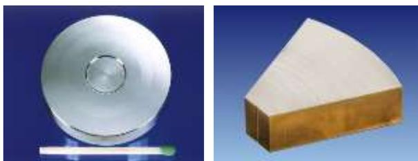
**Figure 1.** Typical roughness standards manufactured at PTB. Left: turned disc. Right: cut and marked roughness standard.
