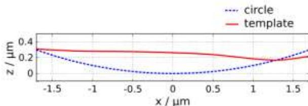
Figure 4. Geometry of the cutting edge used for morphological operation, erosion, as a structuring element: ideally circular (blue dotted curve) and template deduced from measured profiles (red solid curve).
