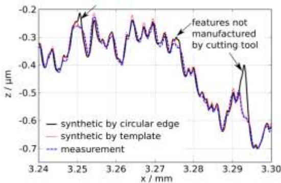
Figure 3. Radial profile on calibration artefact: detail of figure 1.
