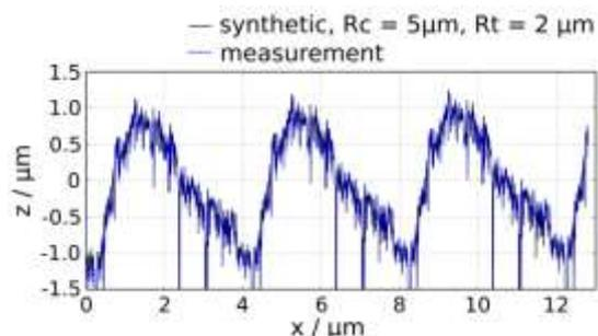
**Figure 2.** Radial profile on calibration artefact: simulated data obtained with ideally circular cutting edge (black solid curve,  $r_c=5\ \mu\text{m}$ ,  $r_t=2\ \mu\text{m}$ ); radially scanned profile (blue dashed curve).
