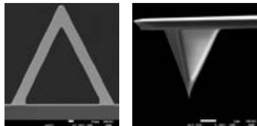
Figure 2. SEM micrographs of Bruker SNL- 10 D SPM probes.
