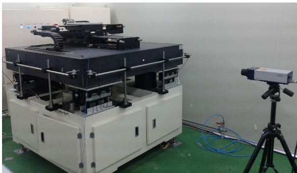
Figure 3. Simulated manufacturing machine on the hybrid mounts and a laser vibrometer
