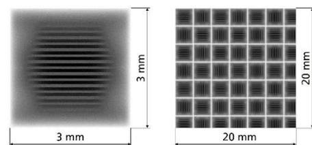
**Figure 1.** Left: Example of an eight bit grey scale bitmap. Pillow structure with subtleties in the dimension of 3x3 mm<sup>2</sup>. Right: Repetitive pillow structure with subtleties in the dimension of 20x20 mm<sup>2</sup>.
