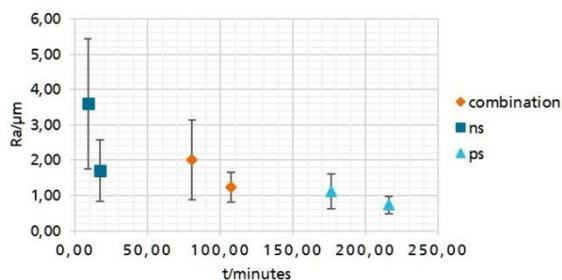
**Figure 2.** Surface qualities ( $R_a/\mu\text{m}$ ) of each process in relation to the processing time ( $t/\text{minutes}$ ) on hot-working steel blanks 1.2311.
