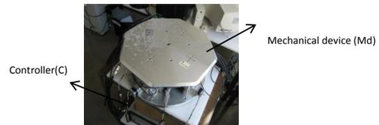
capability to perform maximum: translations -  $X=Y=50\text{mm}, Z=29\text{mm}$  and orientations -  $R_x=R_y=10^\circ, R_z=18^\circ$  with  $3.1\mu\text{m}/20\text{mm}$  and  $2.6 \text{ arcsec}/5^\circ$  accuracy and carrying 100kg load.
