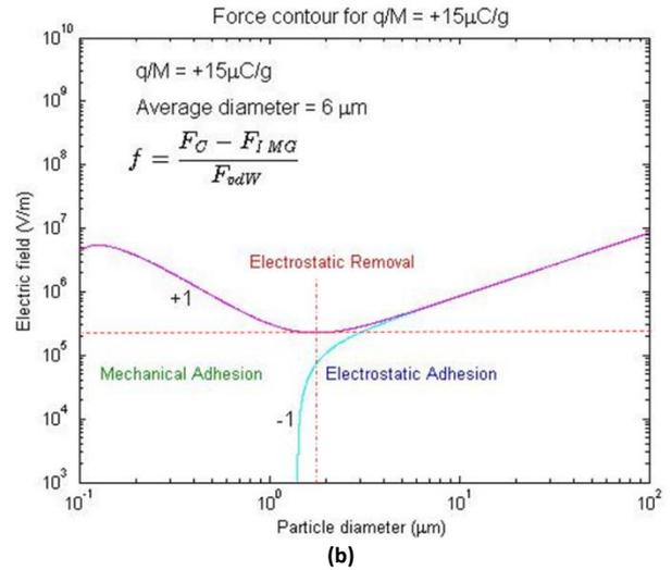
**Figure 3. Equi-force contour graph of (a) the particle of  $-27 \mu\text{C/g}$  and of (b) the particle of  $+15 \mu\text{C/g}$ .**
