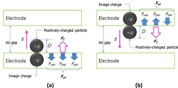
Figure 1. Adhesion and detachment forces when a positively-charged particle is (a) on bottom electrode and (b) under top electrode.
