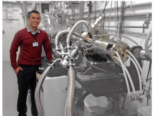
Figure 5. Heat load chopper at BioCARS installed in Sector 14 of the Advanced Photon Source at Argonne National Laboratory.
